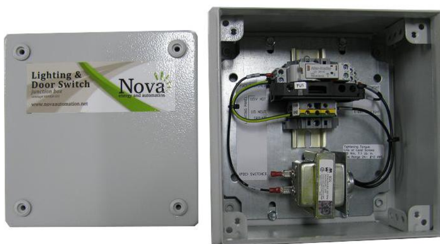
Figure 2: Nova Warning Light Controller- Cover Removed, Inside View
