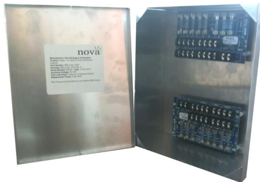
Figure 3: MRI LED Class 2 Power Distribution
